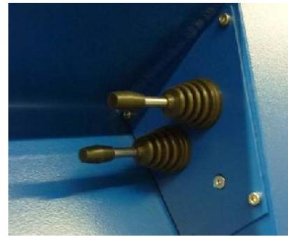
Each straightening unit is equipped with 9 straightening rollers for the processing of twin-strand. All rollers have VV-groove for perfect straightening of round, square or octagonal wire profiles. The last roller of each straightening unit is divided, so that it is possible to adjust the two wires automatically by means of two electronic motors via 2 joysticks during production.
