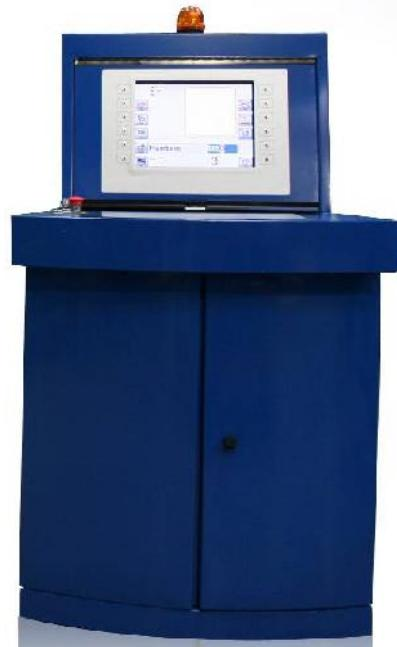
Portable and fixed operating elements for all manual functions are located on the operating console.
